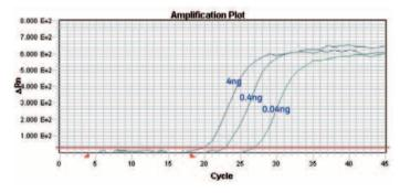
**Fig 5.** The RNAspin Mini Kit total RNA product performs well in sensitive downstream applications such as QRT-PCR. Titration of an RNAspin Mini total RNA sample (NAP274) with TAQ100 primer/probe set (rat thyroid hormone sulfotransferase, ST1B1 gene). (A) QRT-PCR standard curve indicating the appropriate 10-fold differences in the reaction dilutions; (B) QRT-PCT  $C_T$  curves, showing typical response curves for clean RNA template.
