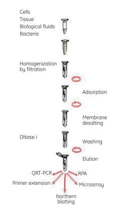
Fig 1. Schematic representation of the RNAspin Mini Isolation Kit protocol.
